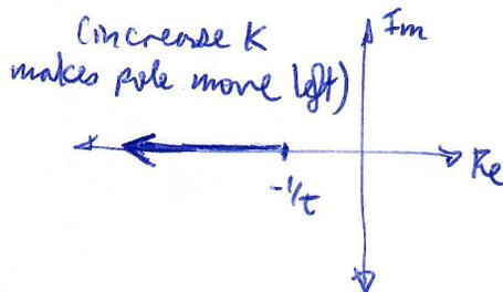
$$\left\{ \begin{aligned} \text{Second example: } G(s) &= \frac{W_n^2}{s^2 + 2\zeta W_n s + W_n^2} \\ C(s) &= K \\ \frac{GC}{1+GC} &= \frac{K W_n^2}{s^2 + 2\zeta W_n s + (K+1)W_n^2} \end{aligned} \right.$$
